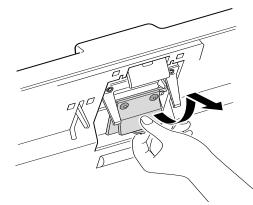
**3** Insert the tabs at the top of the new ADF rubber assembly into the slots and then push it down until it locks into place.
